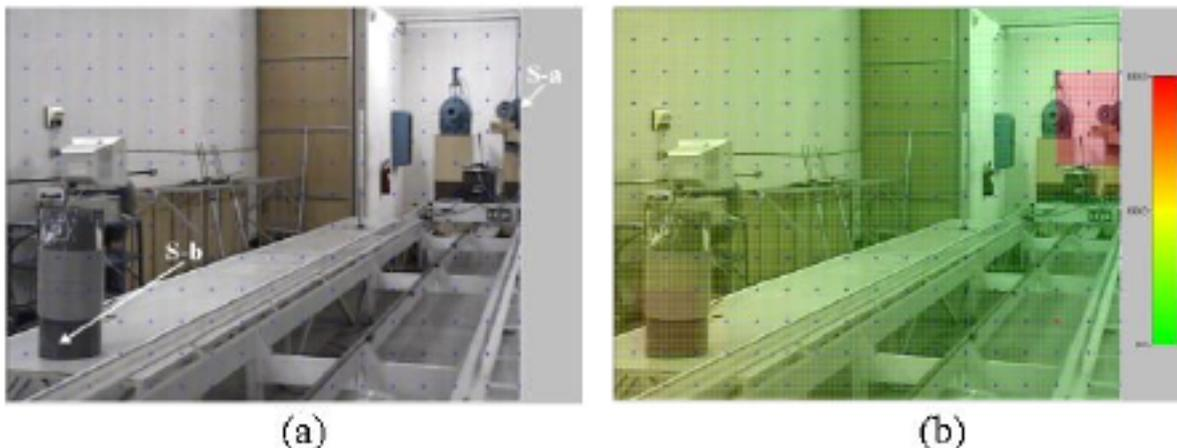
Fig. 4. (a) View of the laboratory used for testing the EDR scanner. (b) Same view colored according with total count rate detected. Color scale adjusted linearly between 0 cps (green) and 800 cps (red).
