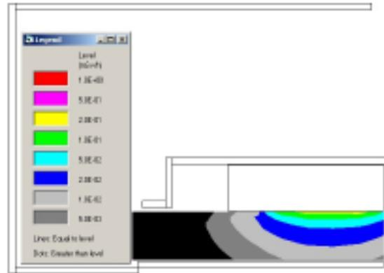
Fig. 4 : Estimation of dose rates inside the cell, via a grid, at the working place
