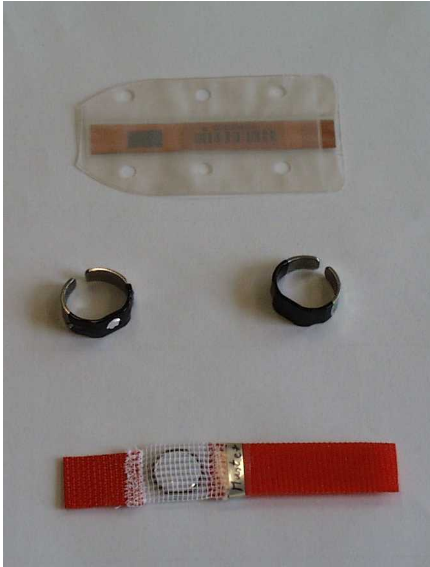
Figure 1: Examples of beta particle dosimeters (partial-body) (from top to bottom: TD1, TD3, TD4, TD5)
