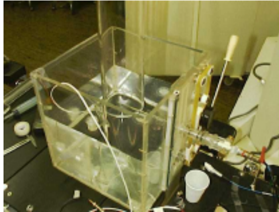
Figure 6. Experimental set-up for the determination of the percentage depth dose curves (PDD), of the practical range ( R_p ) and of the actual energy of the electron beams
