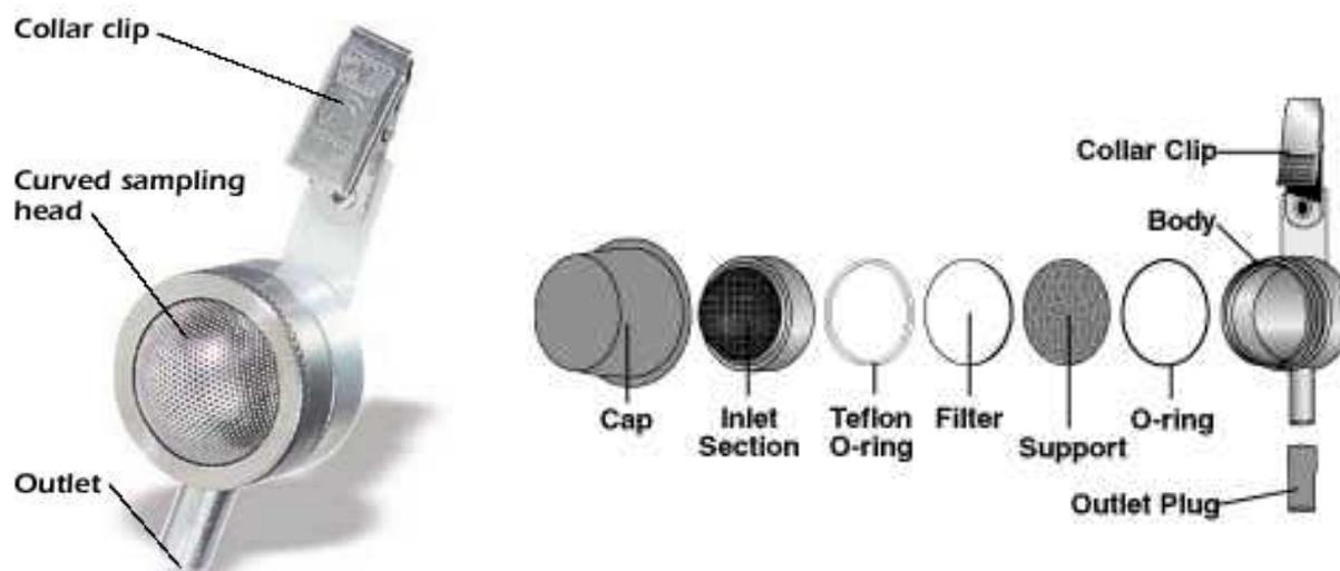
**Figure 7** : General and exploded view of the "Button Personal" aerosol sampler for inhalable dust sampling. Designed by the Department of Environmental Health of the University of Cincinnati (Kalatoor *et al.*, 1995).
