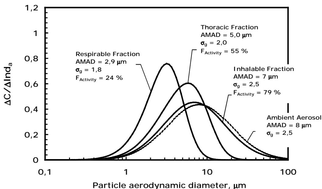
**Figure 2 :** Particle-size distributions and normalised concentrations for the four fractions (i.e. total, inhalable, thoracic, respirable) assuming a log-normal particle size distribution for the total ambient aerosol.
