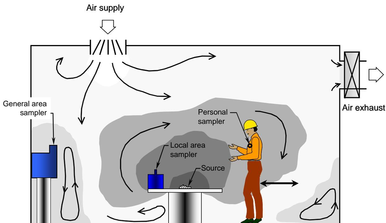
**Figure 4** : Illustration of the particulate contaminant dispersion in a ventilated laboratory and the vicinity of a worker. The nature of the aerosol transport and the sampling performances of the samplers account for differences that are usually measured.
