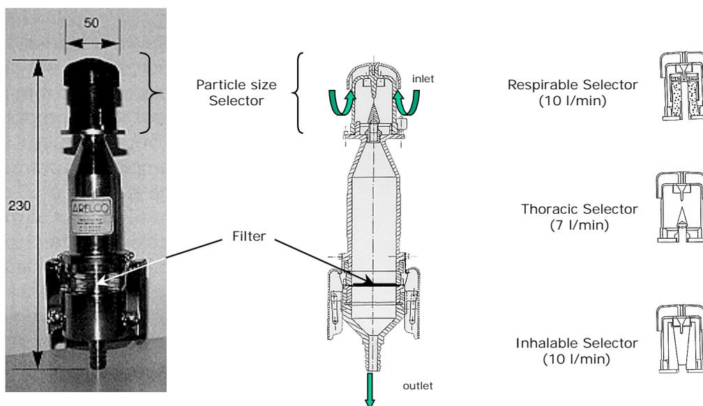
**Figure 6** : General view and schematic diagram of the CATHIA static sampler and the different available particle size selectors for the inhalable, thoracic and respirable fractions. Developed by INRS, France
