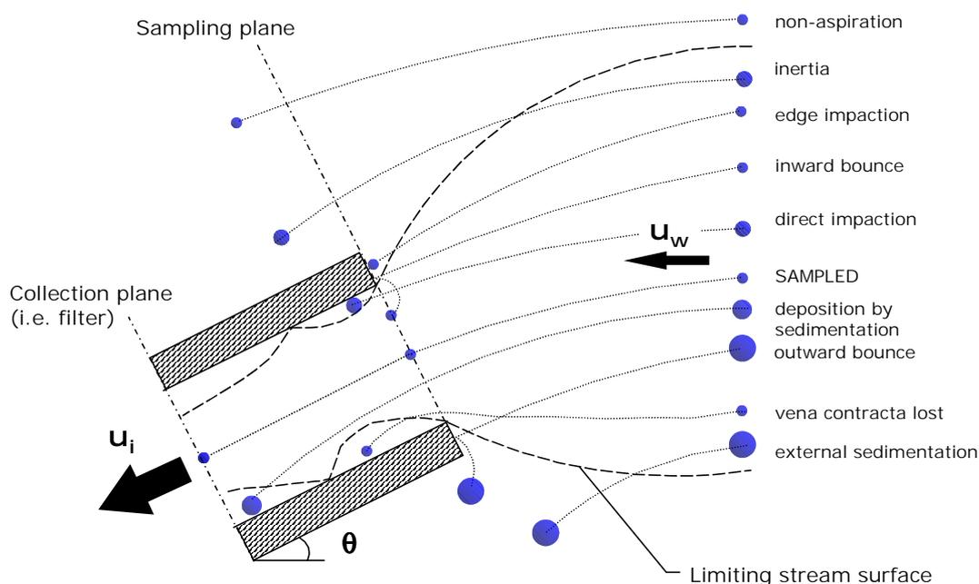
**Figure 3** : Schematic representation of the mechanisms that affect the overall efficiency of a sampling inlet.
