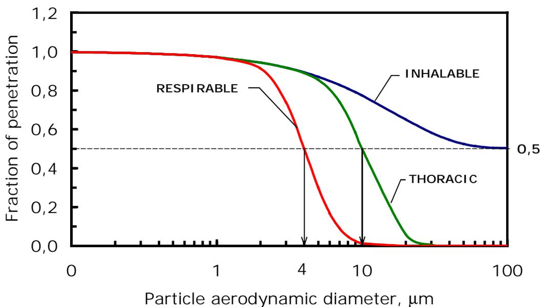
**Figure 1** : Particle size fractions (i.e. inhalable, thoracic, respirable) for health-related sampling in workplaces that have been internationally agreed by CEN, ISO and ACGIH.
