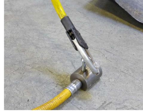
5. Pull at the guide tube in order to move the source into the container.
