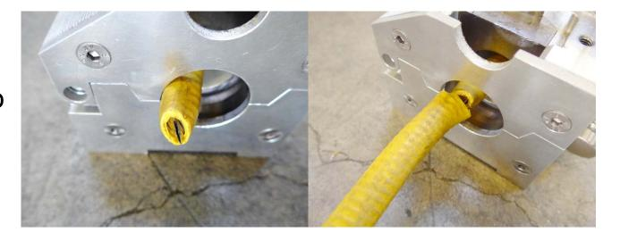
9. Insert the lead shield piece.
