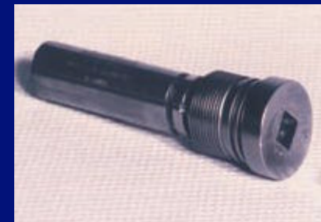
Am-241/Be neutron source for oil well logging
