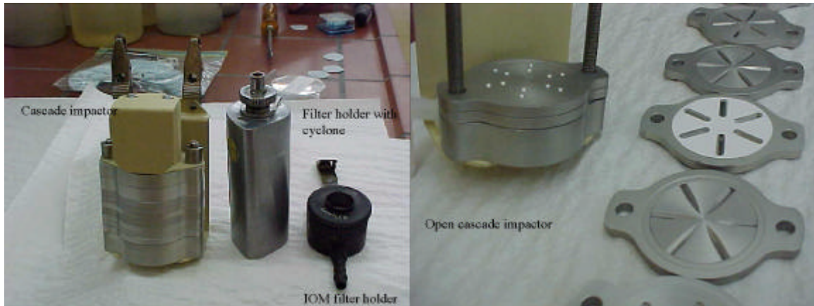
Photos 2 and 3. Filter holders and open cascade-impactor.
