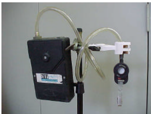
Photo 1. Air pump and IOM filter holder with filter.
