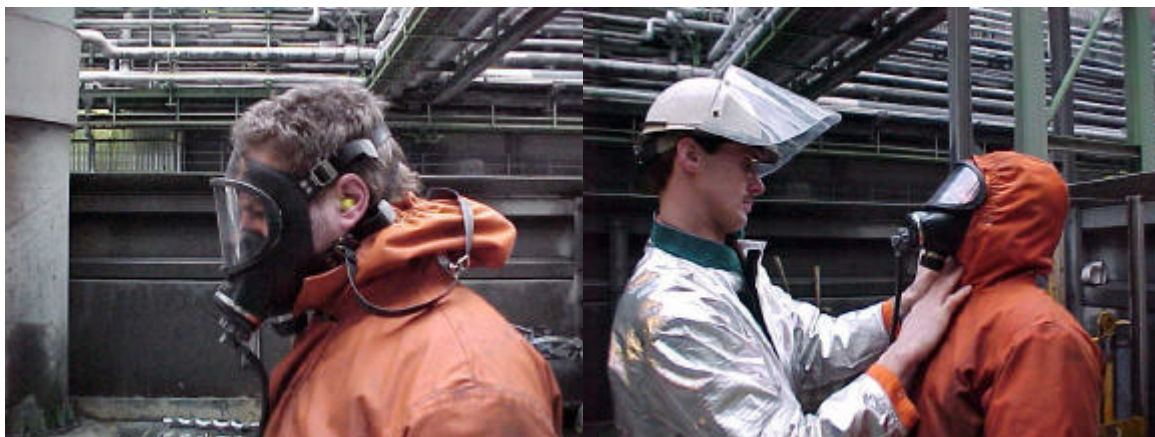
Photos 9 and 10. Full-face mask with remote air supply.
