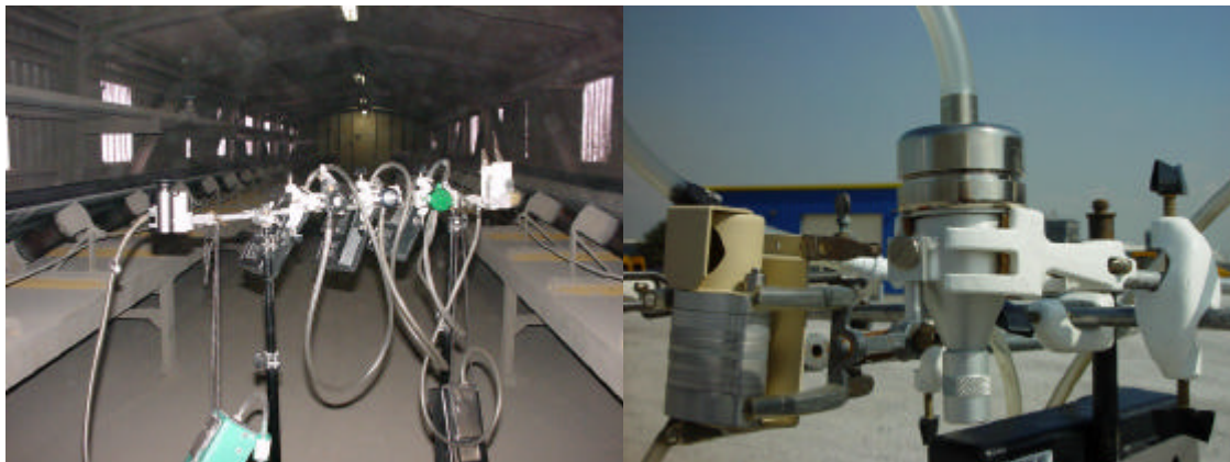
Photos 5 and 6. On the left is a joint measurement setup comprising various measuring devices. On the right is the assembled cascade impactor and a thoracic cyclone.
