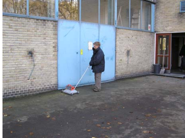
Figure 29. The measurement with a contamination monitor on the area north of the building.
