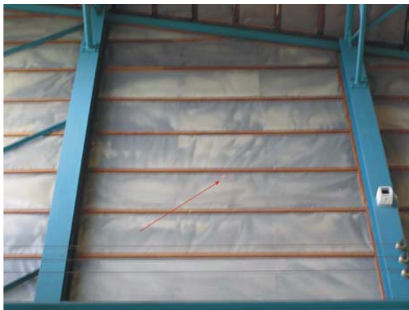
Figure 26. A laser beam is used to position the detector at the western part of the northern wall.
