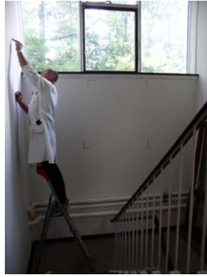
Figure 14. A surface of one square meter is marked on the wall of the stairway.
