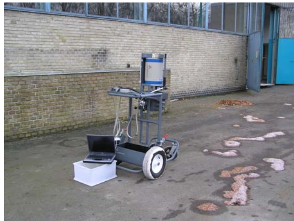
Figure 30. Gamma-spectrometric measurement at the asphalt area north of the building.
