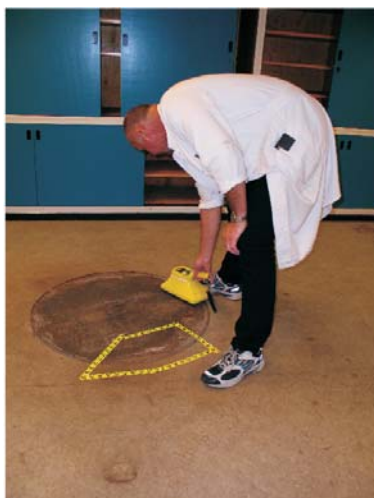
Figure 12. The contaminated area in the counting laboratory. It is clearly seen, where the barrel for the 4\pi -counter was situated.
