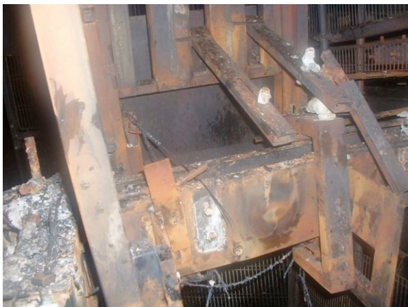
Figure 3. Remnants of the Heuft fill-height detection system
