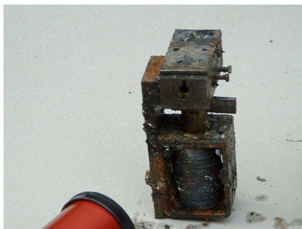
Figure 5. Front view of the recovered component which included the source block containing the Americium-241 source.
