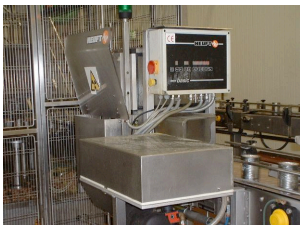
Figure 1. Heuft fill-height detection system (Model Basic 4) on the production line of the plant (pre-fire)
