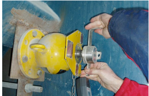
Figure 2: For security reasons the gauge is not usually padlocked in open position, and with the pin grinded off the source holder is easily removed from the shielding.
