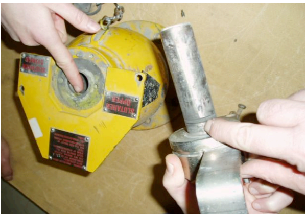
Figure 1: The pin (~5mm) securing the locking mechanism to a slit in the source housing was grinded off.
