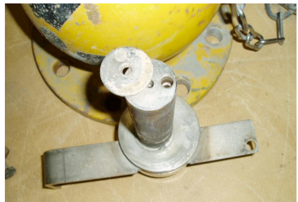
Figure 3: The gauge with the missing source also missed the screw keeping the spring-loaded plate in place.
