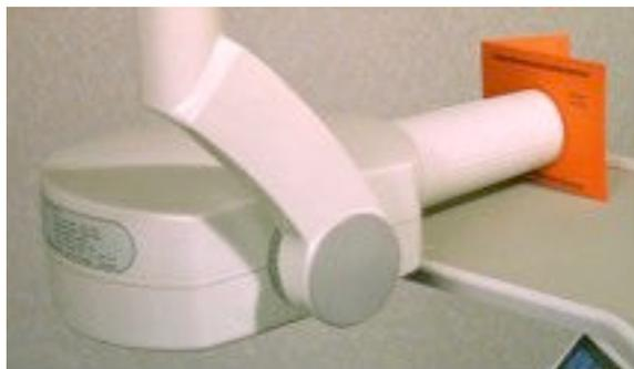
**Figure 1 Exposure of an intra-oral test cassette**
