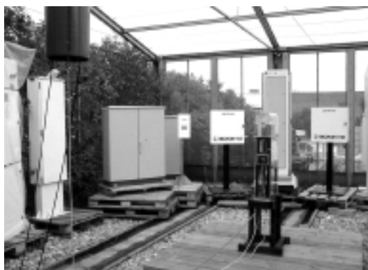
Fig. 2: View of monitoring systems at the lab test facility and the gamma test source (center)
