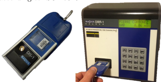
Figure 2. Left panel: Electronic personal dosimeter DIS-1 with integrated neutron dosimeter. Right panel: Reader station.
