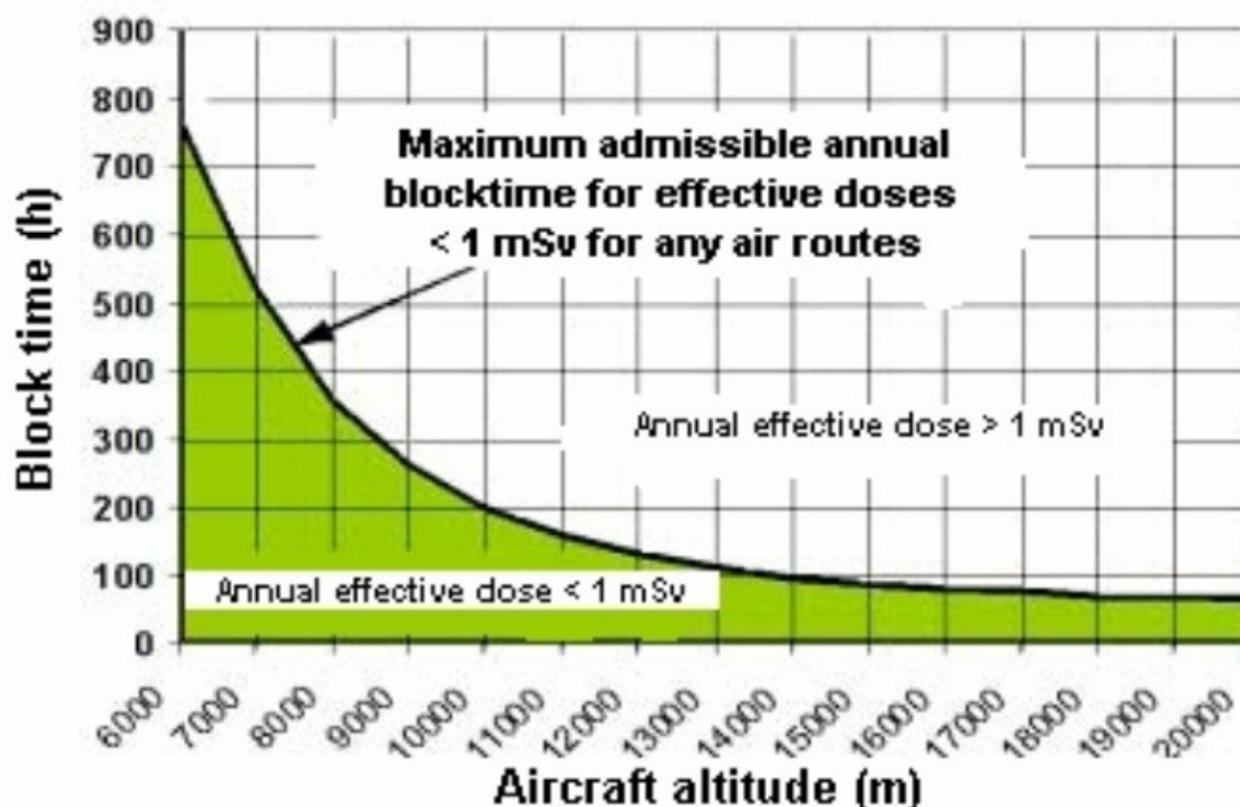
Figure 1: Limiting curve for the keeping of 1 mSv in dependence of the maximum permissible flight hours (block time) and the cruising altitude of the aircraft (Source: Physikalisch-Technische Bundesanstalt, Germany)
