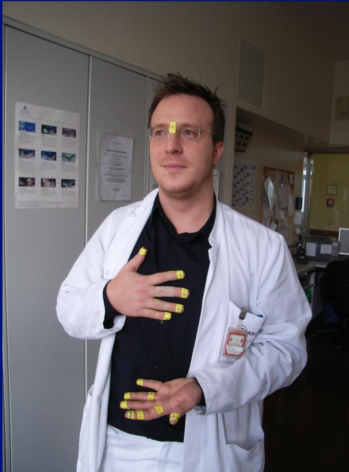
Thin-layer thermoluminescence detectors (TLD)
