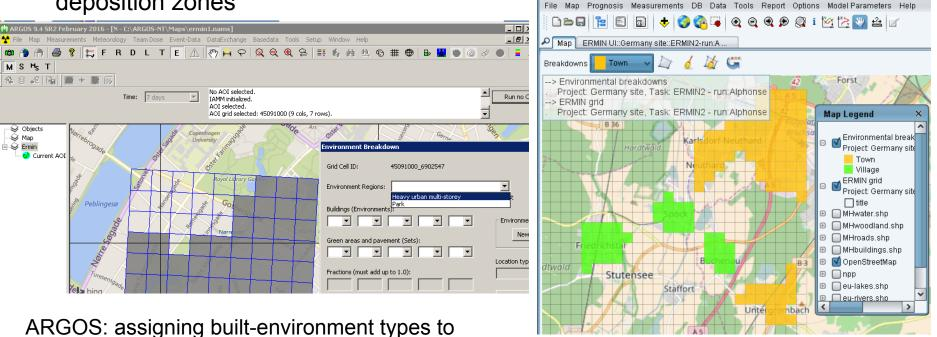
**iRODOS**: assigning built-environment types to model grid squares
