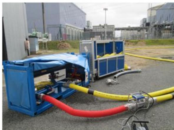
Filter with mechanical auto-cleaning device : 100 microns
