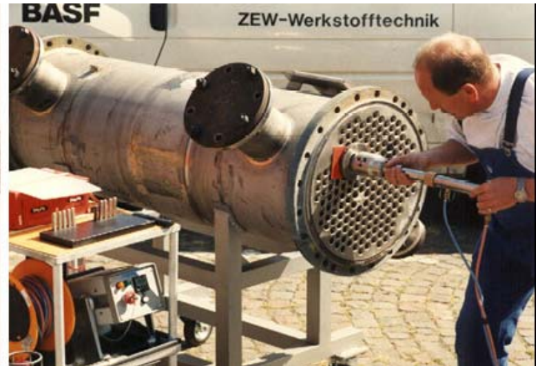
Gammamat B3 isotope source with film holder (left side) at inspection position and set-up for inspection of a small heat exchanger in the field (right side) (Reference: Zscherpel et.al., WCNDT 2008)
