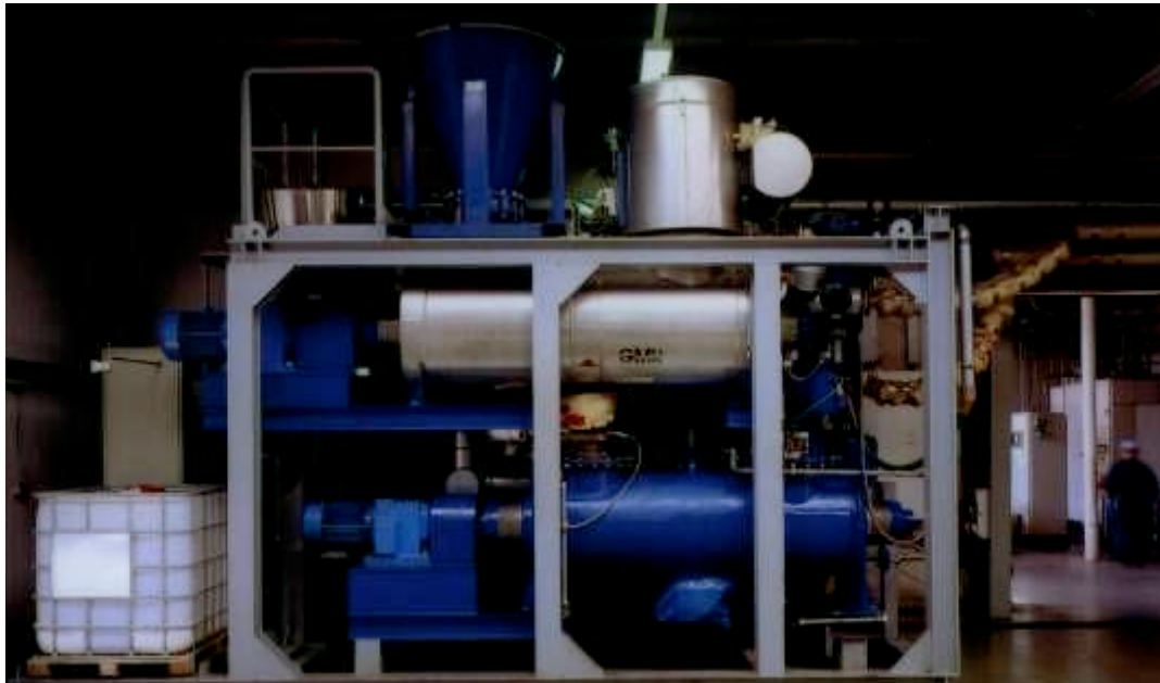
Facility for extraction of raw-mercury by evaporation, condensation and purification (GMR Leipzig)
