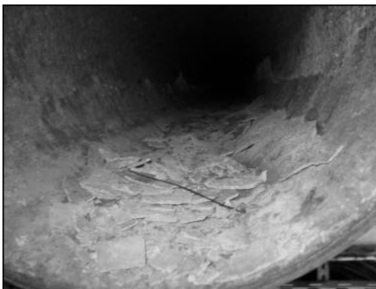
Figure 1. Flakes of LSA Scale in an opened oil production tube.
