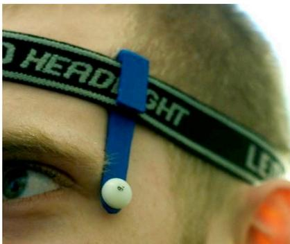
Figure 2. Eye-lens dosimeter
