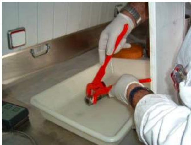
Figure 1. Removal of an Am-Be source keeping inside a Cs-137 source of a density and moisture measurement equipment
