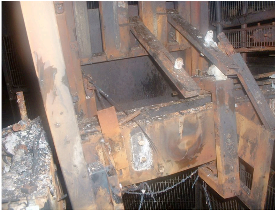
Figure 3. Remnants of the Heuft fill-height detection system
