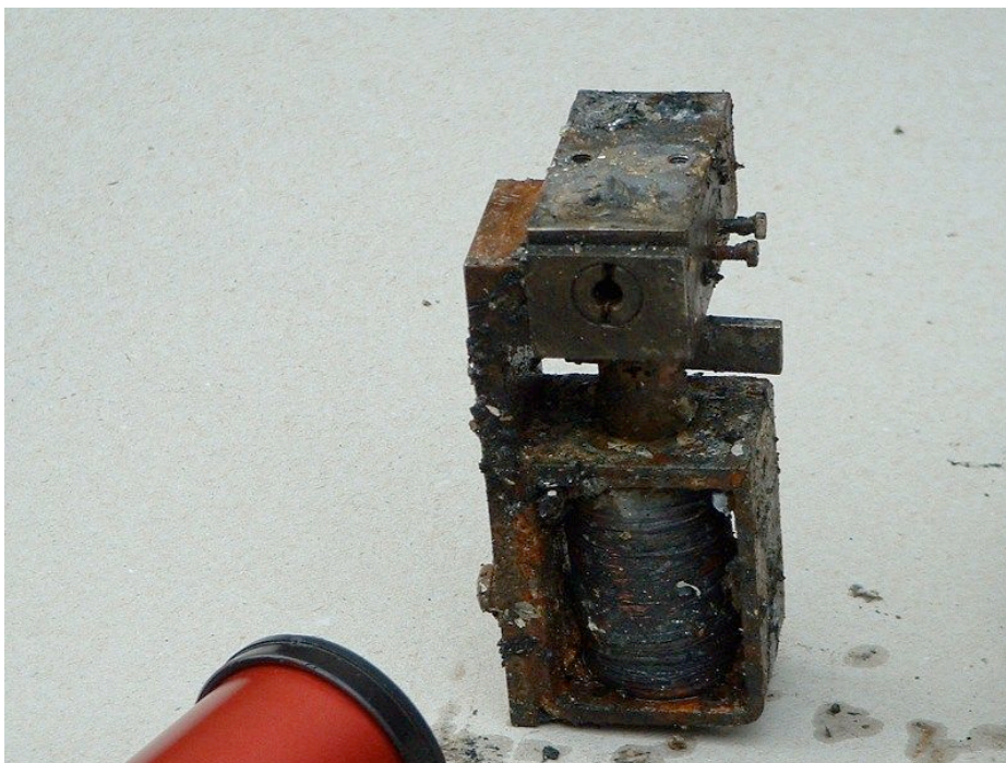
Figure 5. Front view of the recovered component which included the source block containing the Americium-241 source.
