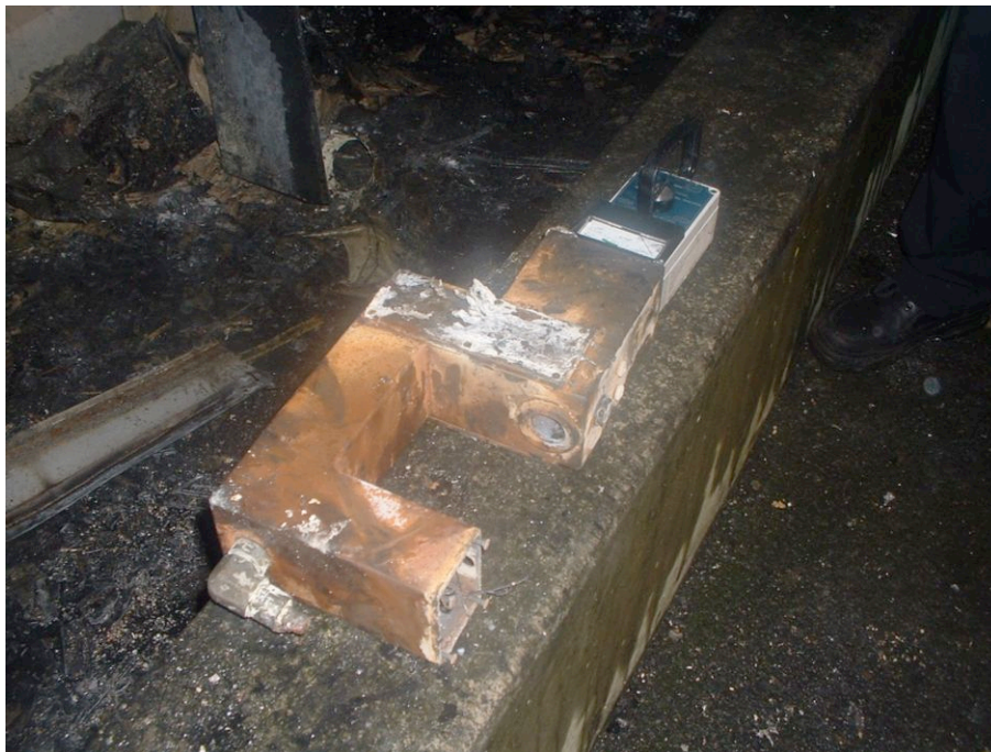
Figure 4. Damaged bridge unit being surveyed outside the building
