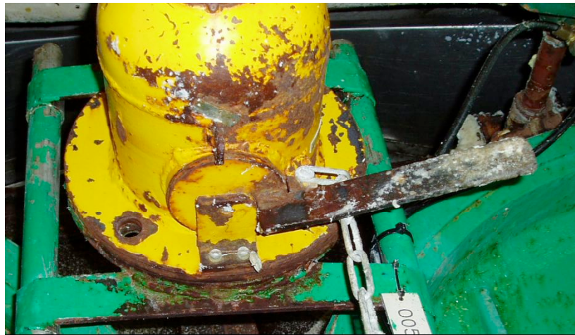
Figure 4: Rusty radionuclide gauge with extended handle
