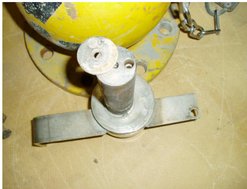
Figure 3: The gauge with the missing source also missed the screw keeping the spring-loaded plate in place.
